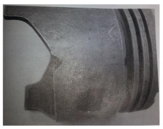
Figure 6.1: Cracked piston
