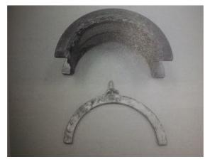
Figure 6.0A: Thrust bearing that has melted on a side
