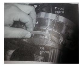
Figure 6.0C: Thrust insert or washer is installed next to the main bearing
